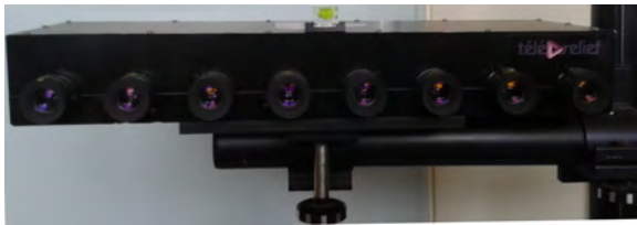
Figure 2: The Octo-cam multiview Camera prototype.
