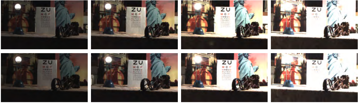
Figure 1: Set of LDR multi-view images taken with an eight view camera using natural color filters to control exposures.
